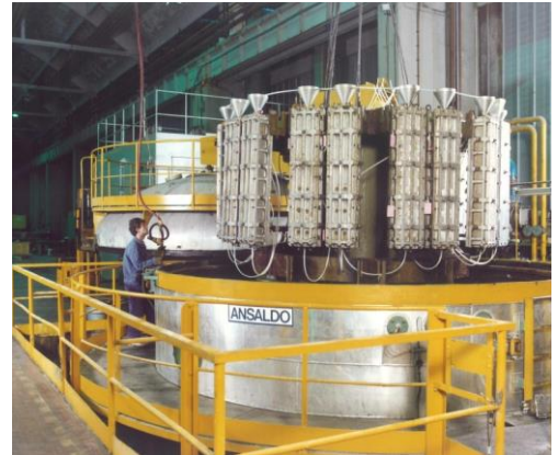
Insertion of the coil moulds in autoclave for curing
